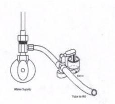
Images in this picture: Water supply, the FLK-14 and Reverse osmosis tubing
