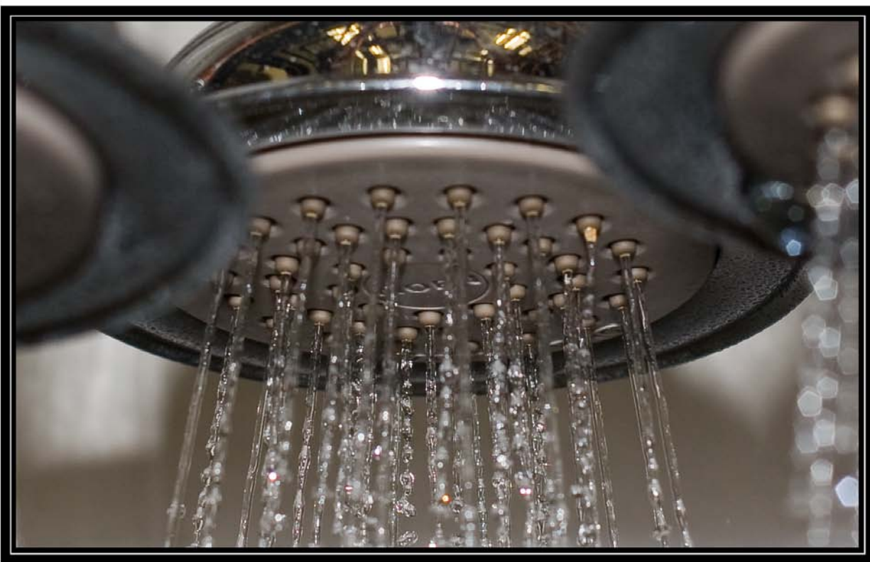
Figure 6-4B. Showerhead 4 on fourth day of testing with softened well water (<1 grains per gallon) showing spray pattern. Battelle testing for Water Quality Association. April 28, 2009
