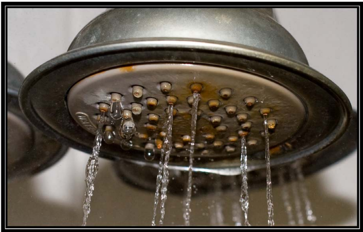
Figure 6-6D. Showerhead 6 on seventh day of testing with hard well water (28 grains per gallon) showing spray pattern. Battelle testing for Water Quality Association. May 1, 2009
