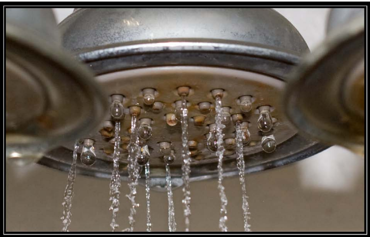
Figure 6-9D. Showerhead 9 on seventh day of testing with hard well water (28 grains per gallon) showing spray pattern. Battelle testing for Water Quality Association. May 1, 2009
