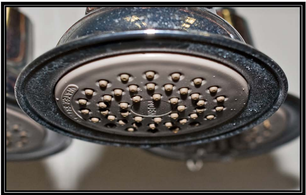
Figure 6-2A. Showerhead 2 on fourth day of testing with softened well water (<1 grains per gallon) showing condition of nozzles. Battelle testing for Water Quality Association. April 28, 2009
